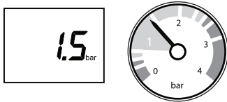
Fig.52 Restore water pressure
