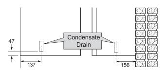
This appliance is fitted with a siphonic 75mm condensate trap system that requires filling before operating the appliance for the 1st time or after maintenance.
