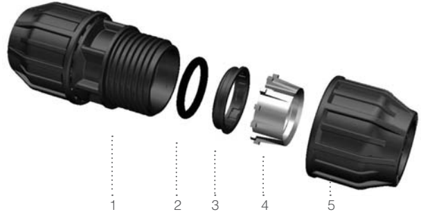
1. BODY - Polypropylene PP-B / 2. O-RING - Nitrile Rubber (NBR 70) / 3. INSERT - Polypropylene PP-B / 4. SPLIT RING - Polyacetal / 5. NUT - Polypropylene PP-B
