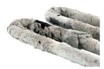
The effects of hard water on an element.
